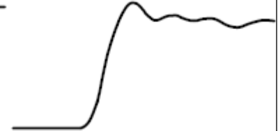
Signal with a long ground lead
