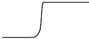
Signal with a short length ground lead
