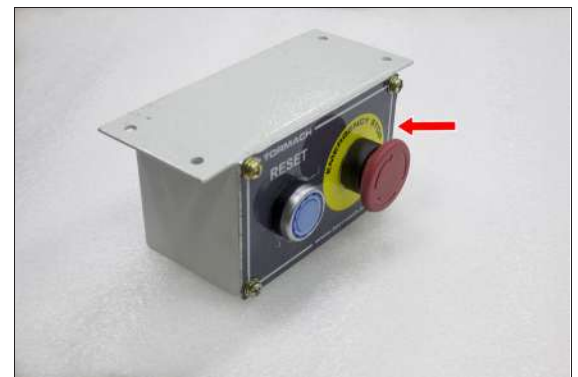
Figure 4-35: Example of the Emergency Stop button locked in the disabled position.
