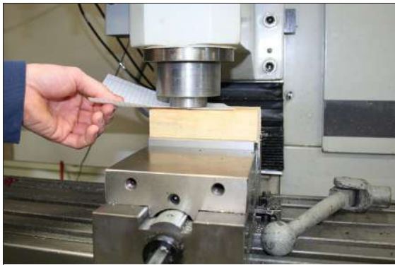
Figure 9-3: Example of using a piece of paper on the workpiece.
