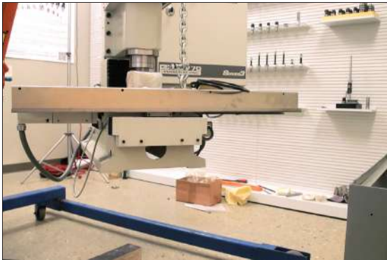
Figure 4-16: Machine lifted parallel to the floor.
