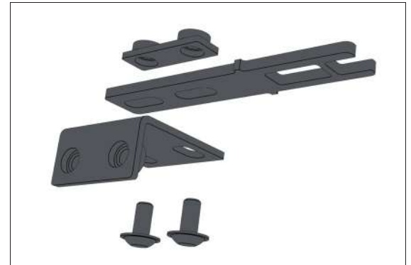
Figure 4-154: Attaching the components of the lock key bracket assembly.
