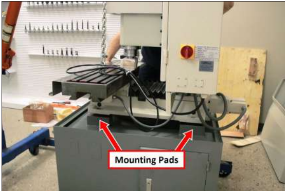
Figure 4-17: Machine lowered on to the mounting pads on the machine stand.
