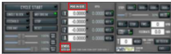
Figure 7-60: Work offset indicated in the PathPilot interface.
