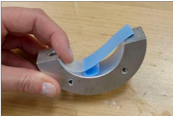
Figure 4-175: Adhering tape on the inside of a split collar.
