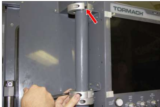
Figure 4-181: Loosely attaching the split collars to the mount arm.
