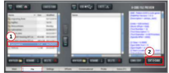
Figure 7-7: Edit G-code button on the File tab.
