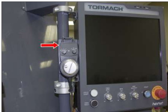
Figure 4-183: Jog pendant on the front of the console assembly.
