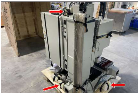
Figure 4-8: Axis motors secured to the pallet.
