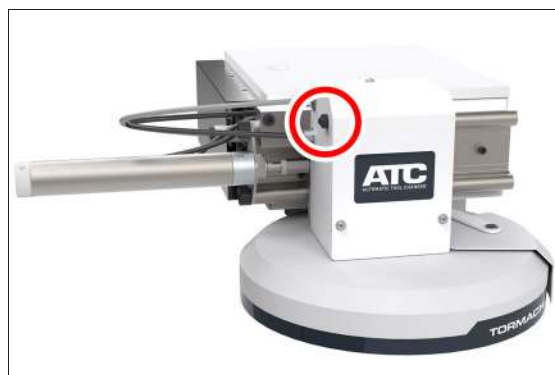
Figure 4-87: Collet open button on the side of the ATC.
