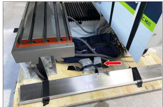
Figure 4-6: Y-axis bellows spacers on the pallet.
