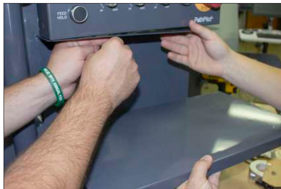
Figure 4-182: Attaching the keyboard tray to the bottom of the controller.
