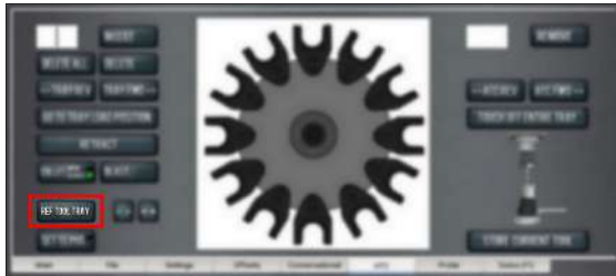
Figure 4-93: Ref Tool Tray button on the ATC tab.
