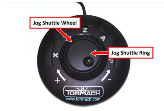
Figure 4-40: Functions on the optional Jog Shuttle.
