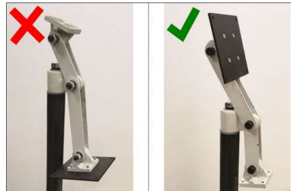
Figure 4-22: Incorrect and correct orientations of the monitor bracket on the Controller Arm.
