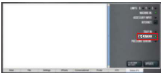
Figure 4-88: VFD Running light on the Status tab.
