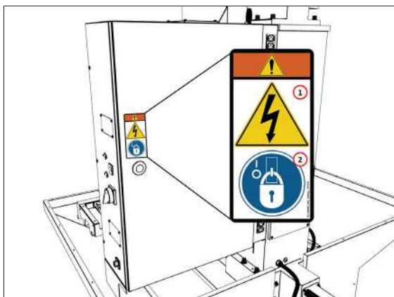
Figure 1-1: Example of a safety decal on the electrical cabinet door.
