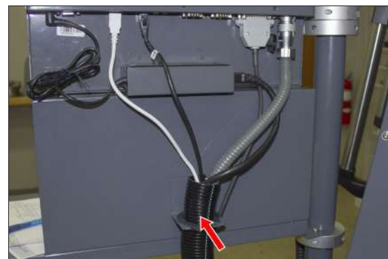
Figure 4-186: Cords put into corrugated tubing, which is attached to the rear of the keyboard tray.
