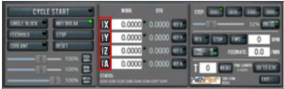
Figure 9-5: Zero X and Zero Y buttons.
