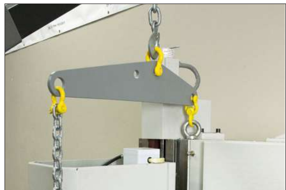
Figure 4-15: Lifting Bar Kit connected to the machine.
