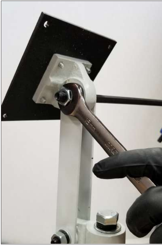
Figure 4-23: Tightening the monitor bracket in place.
