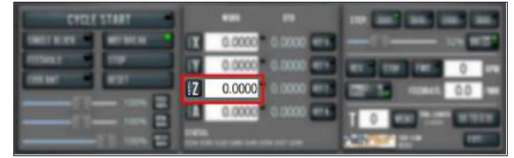
Figure 8-9: Z-axis work offset DRO field.
