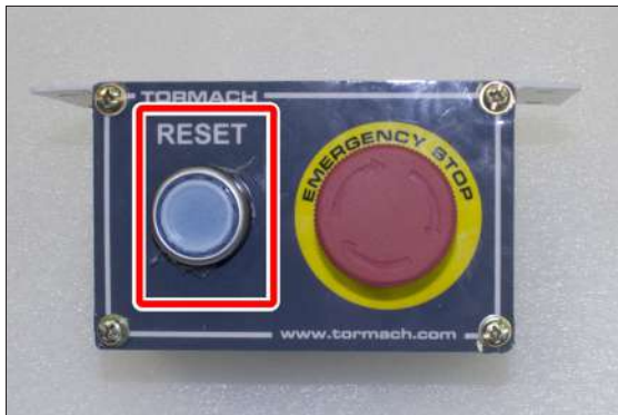
Figure 4-31: The Emergency Stop button on the operator box.
