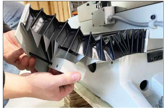
Figure 4-7: Installing the Y-axis bellows spacer.
