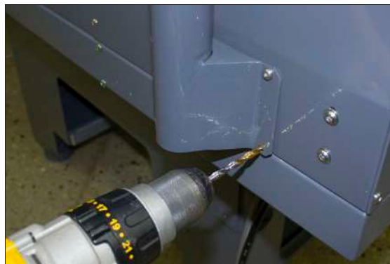
Figure 4-172: Drilling the remaining three holes into the enclosure.
