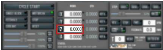
Figure 9-4: Z-axis work offset DRO field.
