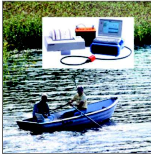
Fig. 7.12 Simrad EY 500 portable scientific sounder system Simrad Company
