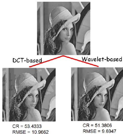
Figure 6.2: Comparison between JPEG and JPEG 2000. CR stands for compression ration and RMSE means root mean square error.
