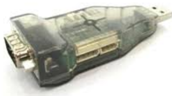
FIGURA 4.3: Conector USB2 Dynamixel.
