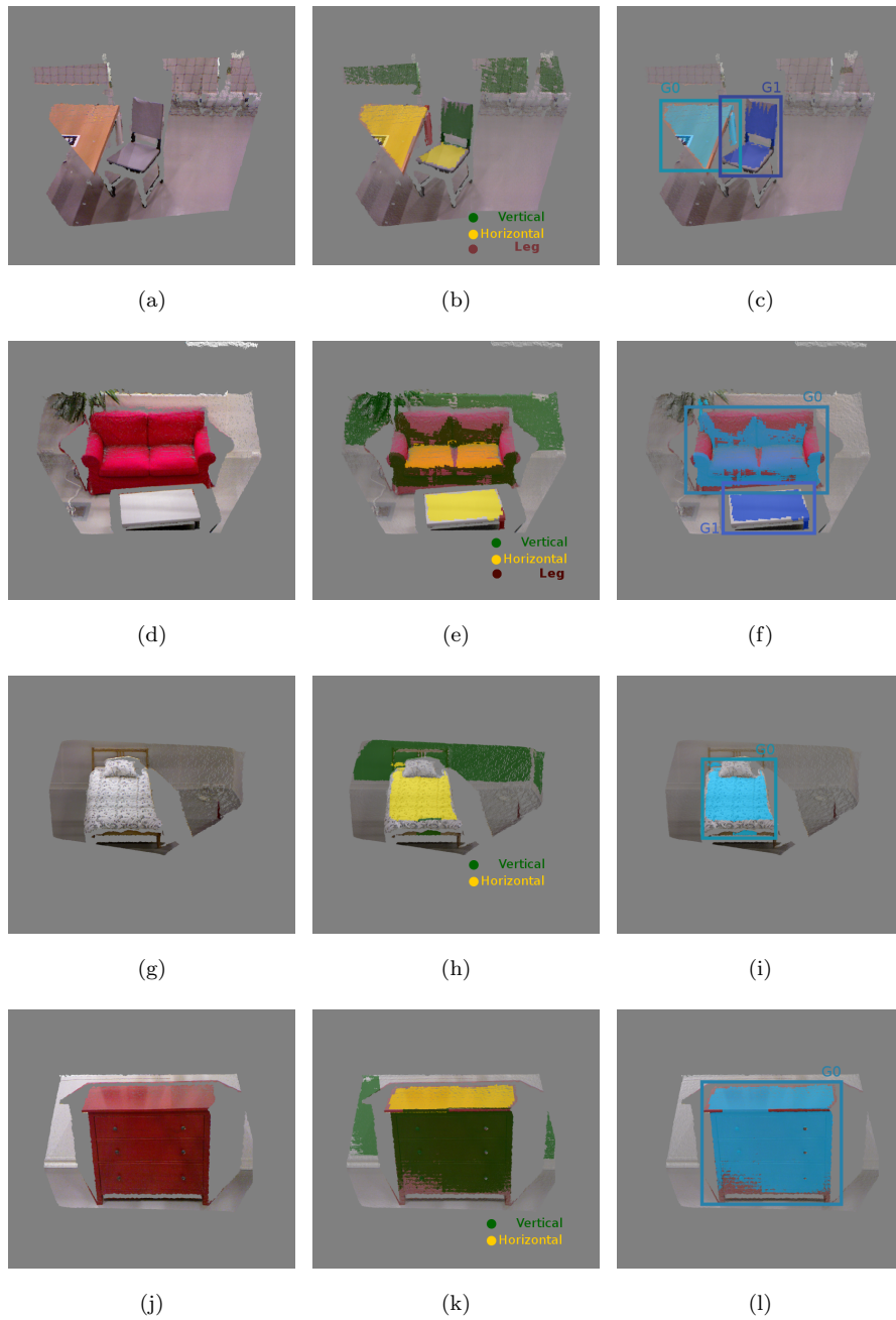
Figure 6.5: Results for the furniture detection, each row shows one scene. In a), d), g) and j) the original point clouds. In b), e), h) and k) are shown the geometric components found, the vertical planes are in color green, the horizontals in yellow and the legs in red. The bounding boxes in c), f), i) and l) show the graph generated that were correctly identified as a piece of furniture
