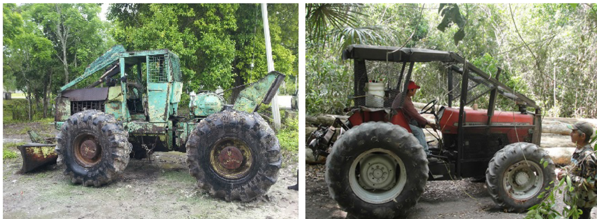
Fig. 2. A forestry skidder (left) and a modified agricultural tractor (right) used for log yarding on the Yucatan Peninsula.
