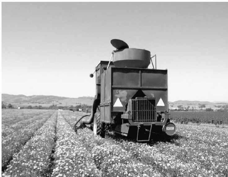
Fig. 11.11. Calendula seed being harvested by a custom-made vacuum harvester.
