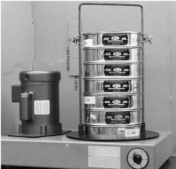
Fig. 12.3. Stacked sizing machine. Screens are stacked vertically from largest to smallest aperture size. As the machine shakes in a circular motion the seed falls through the screen until it reaches a screen with holes too small for it to go through. The seed collected above each screen represents a size fraction approximating to the screen aperture.
