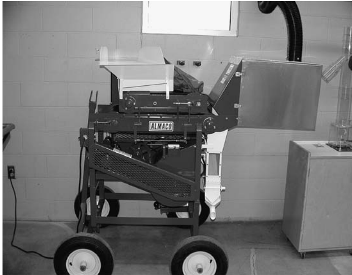
Fig. 17.14. The spring-loaded belt thresher for cleaning bigger seed lots at the Ornamental Plant Germplasm Center.
