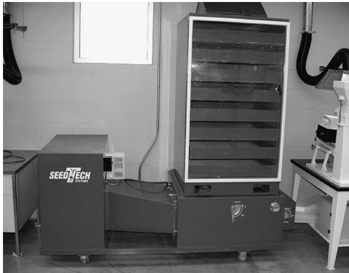
Fig. 17.15. The high volume airflow ventilator/dryer makes use of the dry air-conditioned environments of 25^{\circ}\text{C} and 40%–50% relative humidity for drying wet seed.
