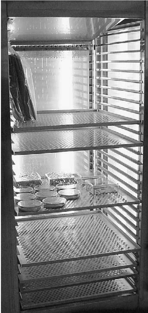
Fig. 14.4. In freestanding germination units, light panels are situated on the sides, back and/or on the inside of the door.
