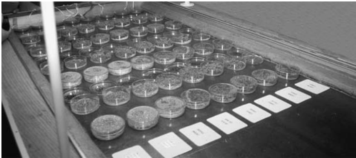
Fig. 16.2. Petri dish germination studies using a thermal gradient table.
