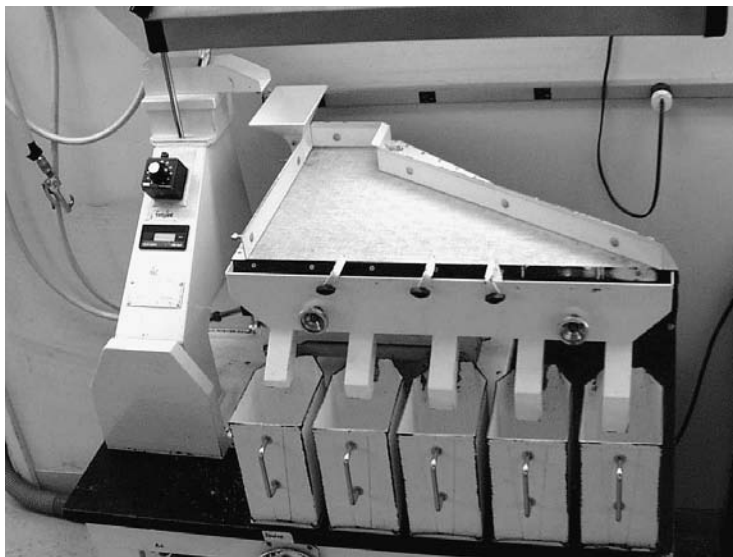
Fig. 12.12. A small gravity separator. The lightest seed is collected in the far left bin and the heaviest seed is collected at the far right. Up to five density fractions can be obtained.
