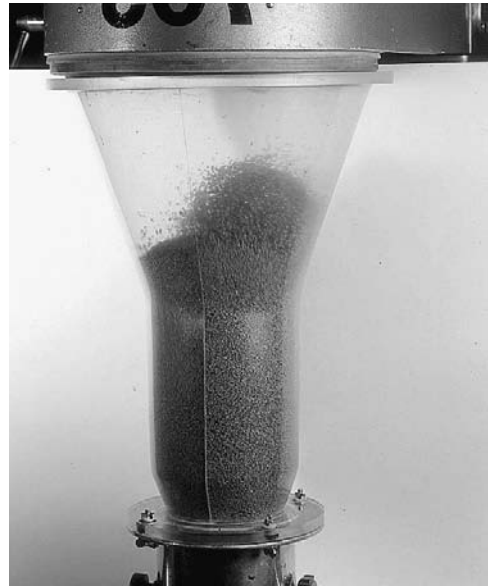
Fig. 13.10. Equipment for film coating according to the fluidized bed method.
