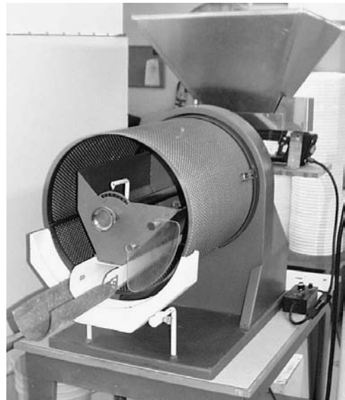
Fig. 12.7. A laboratory size indent cylinder separator commonly used for length separation.
