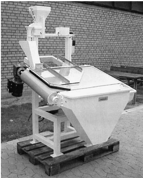
Fig. 12.16. A belt grader manufactured by Westrup (Slagelse, Denmark).
