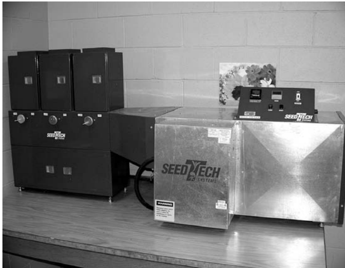
Fig. 17.9. The Ornamental Plant Germplasm Center (OPGC) STS temperature- and time-controlled precision dryer.
