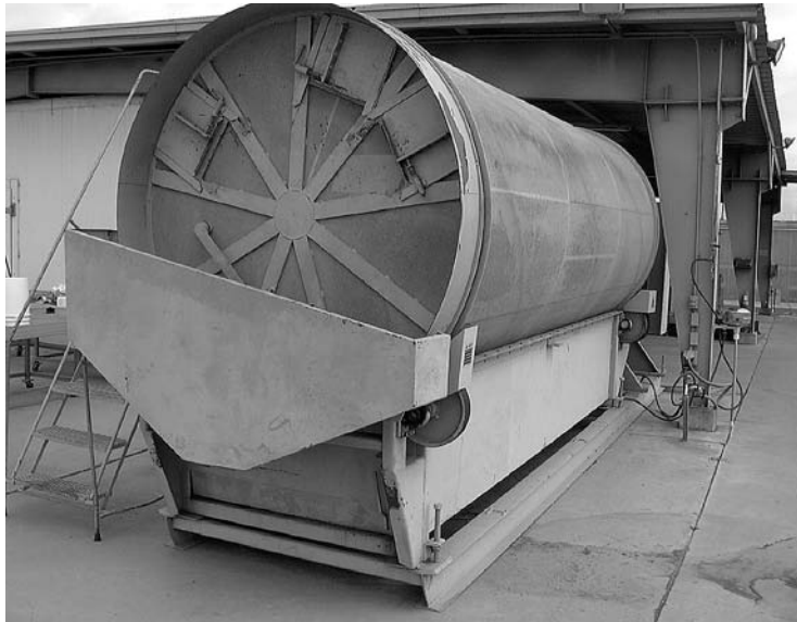
Fig. 11.13. Rotary dryer used for drying plant materials.
