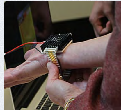
Responsive Bracelet Sends Thermoelectric Pulses To Heat Or Cool A Person's Entire Body
